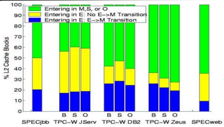
Removing E state would necessitate an extra bus transaction for 9%-28% of all L2 Misses.
