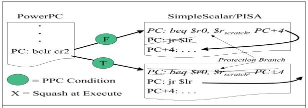
**Figure 2. Illustration of PowerPC** *bclr* **instruction implementation.** Depending on the conditional, the register-direct branch or the protection branch is squashed before it can affect control-related logic.
