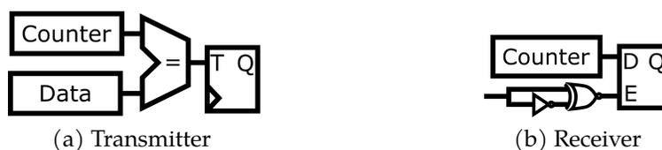
Figure 6.1: Basic Temporal Transmitter and Receiver Designs.
