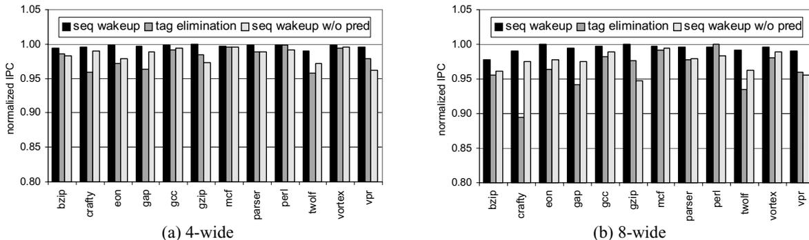
**Figure 14. Performance of sequential wakeup.** Note that sequential wakeup without a predictor outperforms the tag elimination scheme with a predictor in many benchmarks, showing that the misprediction penalty in sequential wakeup is slight.
