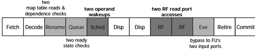
**Figure 1. The base machine model and pipeline stages that handle two source operands.** Instructions with two source operands complicate many stages in the pipeline, which are illustrated as shadowed boxes. This paper discusses possible solutions for the scheduling (Sched) and register file access (RF) stages.
