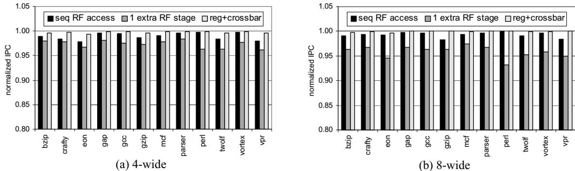
**Figure 15. Performance of sequential register access.** From left to right, sequential register access with one read port per issue slot (*seq RF access*), a conventional register file with one extra pipeline stage (*1 extra RF stage*), and a register file with half the number of read ports + a fully connected crossbar to all functional units (*reg + crossbar*).
