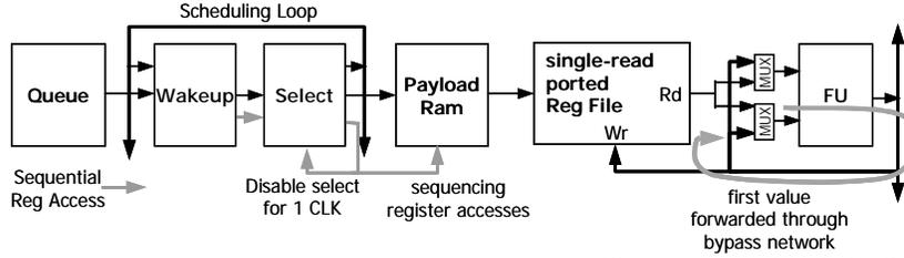
**Figure 13. The changes in the pipeline for sequential register access.** Unlike an conventional pipeline with 2 register read ports per issue slot, the register file has only one register port per issue slot.
