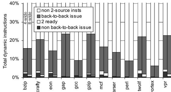
**Figure 10. Characterization of register accesses.** Two stacked bars from the bottom (*non back-to-back issue* + *2 ready*) show that less than 4% of instructions require two port accesses to the register file in most benchmarks.
