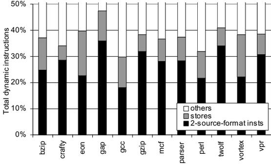
**Figure 2. Percentage of 2-source-format instructions.** 18~36% of instructions have two source operands in their format. Stores are presented in their own category since they are handled differently inside the processor core.
