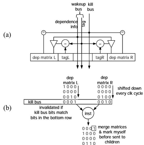
**Figure 5. A possible implementation of selective recovery logic.** (a) the list of issued parent instructions in the pipeline is propagated to dependent instructions along with tag broadcasts. (b) the source operand with matching bits in the kill bus is invalidated, indicating that misscheduling of its parent instruction is detected.
