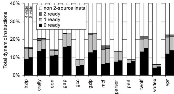
**Figure 4. Breakdown of 2-source instructions, as a function of the number of ready operands when they are inserted into the scheduler. Only 4~16% of instructions have 2 unresolved operands at insert time.**
