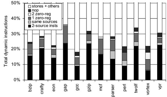
**Figure 3. Breakdown of 2-source-format instructions.** Only instructions in the bottom-most bars have 2 unique source operands that create dependences. They will be referred to as *2-source* instructions in the later sections.
