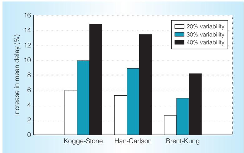
Figure 1. Increase in arithmetic logic unit (ALU) delays due to random variations. Each bar represents the mean delay of a distribution of 1,000 generated circuits.
