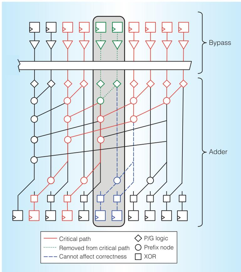
Figure 3. Example of adding two extra bits to an 8-bit Han-Carlson adder. The shaded region indicates the location of the two RIBs.
