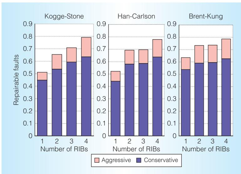
Figure 4. Fraction of repairable adder faults with different numbers of RIBs. Adding more redundancy increases the fault coverage.
