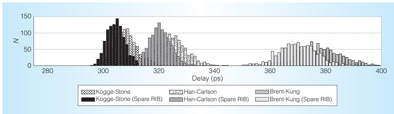
Figure 5. Histograms of ALU critical-path delay. Every distribution comprises 1,000 circuits, each with randomized delays and 40 percent threshold voltage variability. Our scheme with one spare RIB consistently improves the delay distribution.
