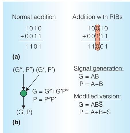
Figure 2. Adder operation with Spare RIBs (redundant intermediate bit slices) and required modifications. Conceptual example of binary addition with RIBs (a). Note that the carry traverses the extra slice. Basic prefix adder operation (b). Our proposal adds an additional skip input  $S$  to the initial propagate and generate logic for each bit position.  $A$  and  $B$  are operand bits at a given offset.
