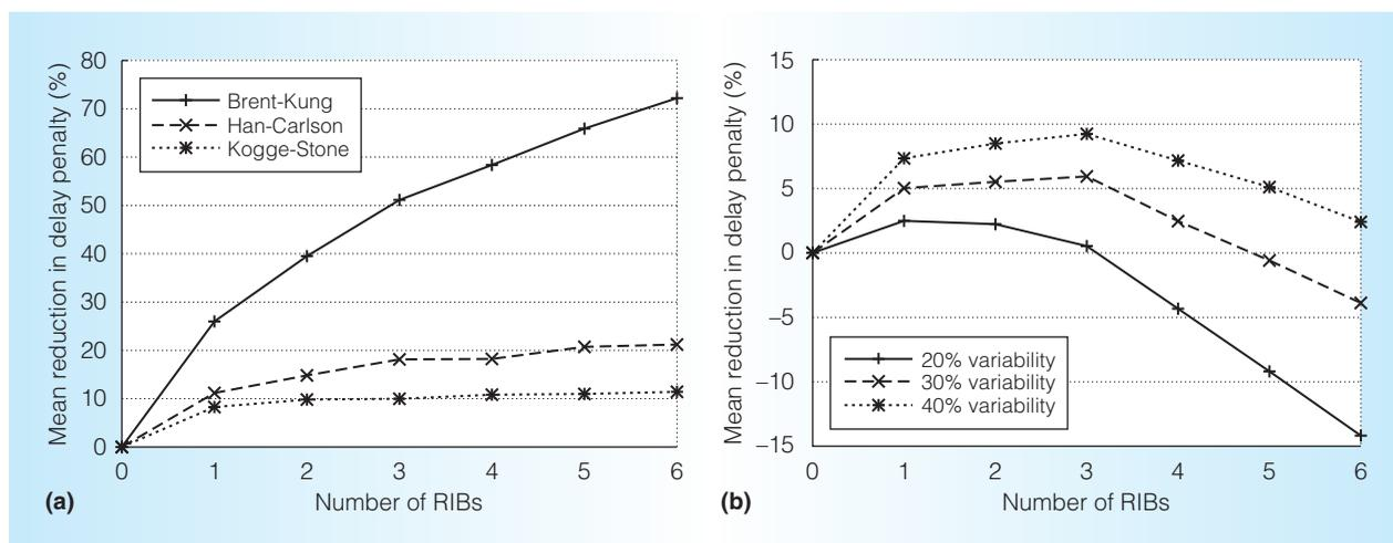
Figure 6. Benefit of RIBs in the ALU (a) and the register file (b). We can reduce the delay penalty incurred by random variations by adding more RIBs. In these experiments, threshold voltage variability is set to 40 percent. For the register file, we see an optimal number of RIBs in terms of the delay reduction.
